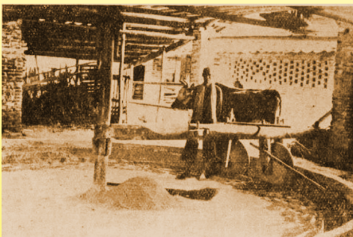
Grinding of kaolin by grinders powered by an ox (1939, Vienam, Economic Bulletin of Indo-China)
