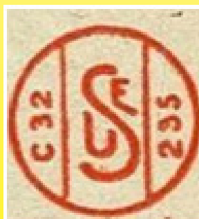
1957 Marking USE printed with the standard number (C32) and the manufacturer identification number (295)
