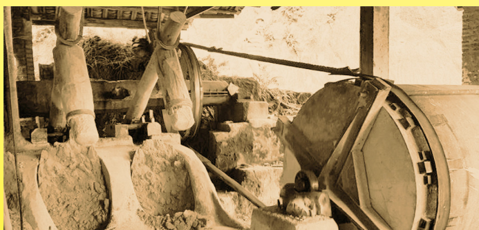
Traditional production machines ((水確 shui dui) for production of powders used to make electric porcelain (private collection)
