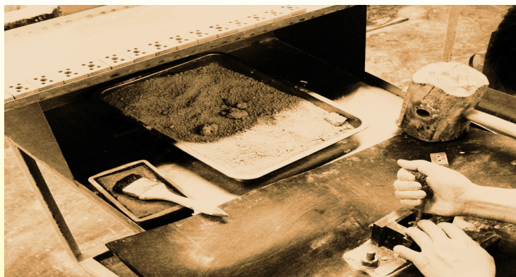
Porcelain Terminal Blocks Hand Made by Hammer Pressing: Manual Filling of Wet Granulate (Private Collection) Drying of Electric Porcelain After Pressing (Private Collection)
